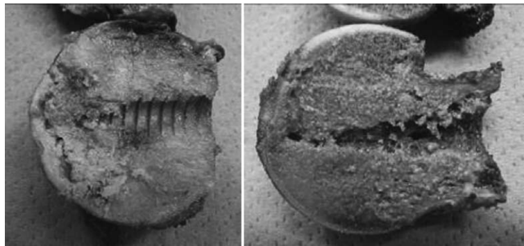
Fig. 2-4. Cross-sectional images of after-test samples (Left : lag screw ; Right : grasping pin) (material : femoral head)
