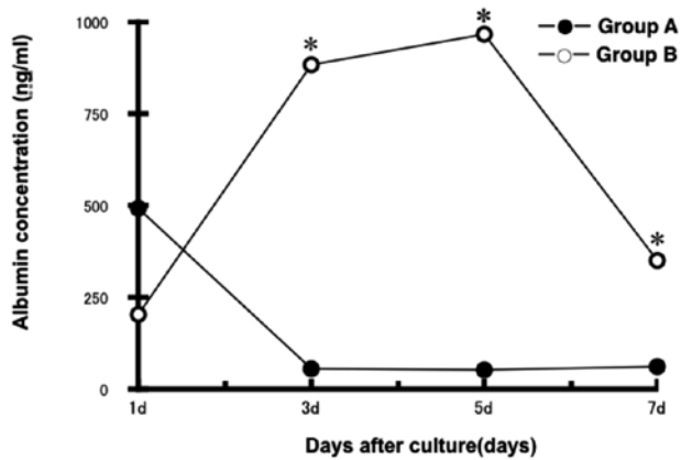
Fig. 2. Albumin production by cells cultured in the RFB and the floating culture system. Data are expressed as mean \pm SD ( n=3 ). Group A: floating culture system, Group B: RFB-PVA culture system. (* P<0.05 compared with Group A).
