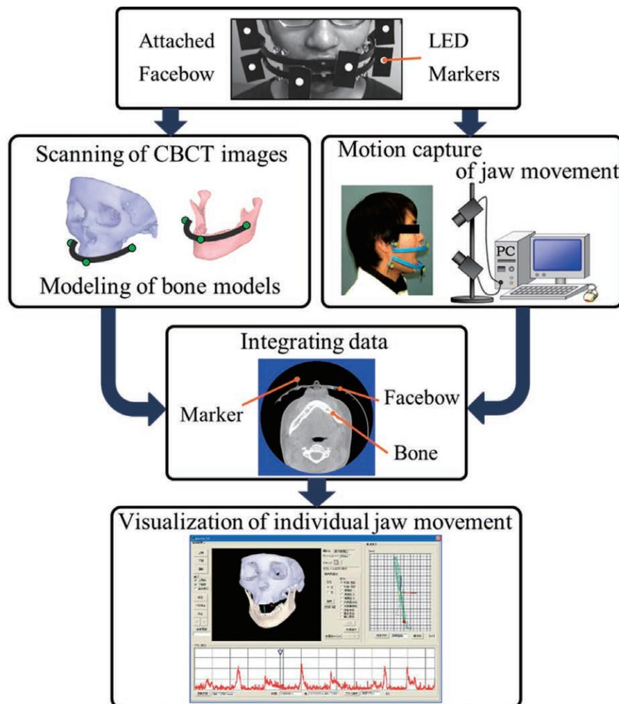
Fig. 1. Diagram of the three-dimensional display system. This shows the procedure up until the display of individuals' jaw movement. This was obtained from the coauthor's manuscripts<sup>11-13</sup>.
