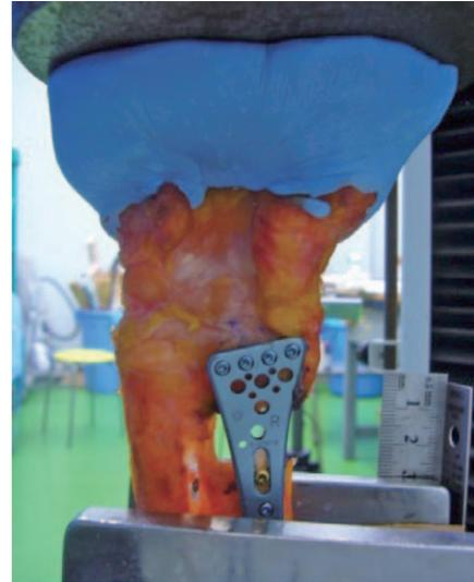
Fig. 4 Experimental setup used for the application of continuous cyclic loading on the cadaveric radius fracture models. Proximal side of the radius molded with poly-methyl methacrylate resin was vertically anchored in a loading machine and the axial load was applied to the distal end of the specimen via a uniform flat surface of poly-methyl methacrylate resin.
